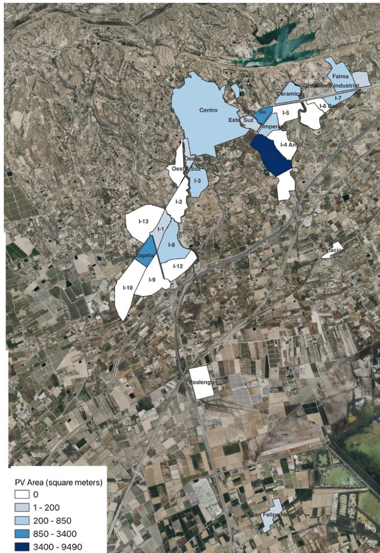
Figure 20. Area of PV installation per zone. Scale 1:40000. Source: Adapted by the author on QGIS.
