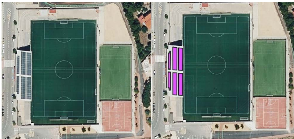
Figure 10. Manual annotation of PV installations at the municipal stadium Source: Adapted by the author on QGIS.
