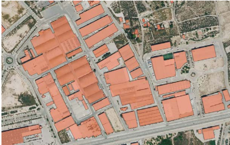
Figure 17. Examples of results of detection of buildings from aerial imagery using Mapflow. Source: Author's elaboration on QGIS.
