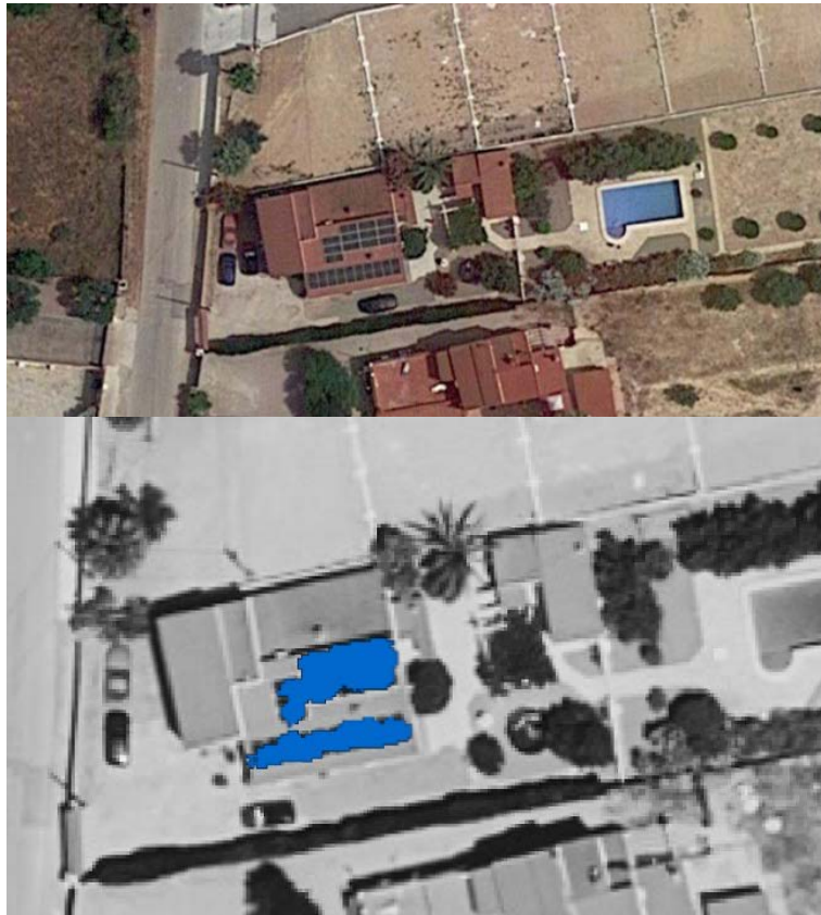
Figure 16. Example of detection of a photovoltaic installations Source: Adapted by the author on GRASS GIS.
